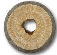
A cross-section of built up lime scale on the outlet of a water heater in Northern Illinois.
