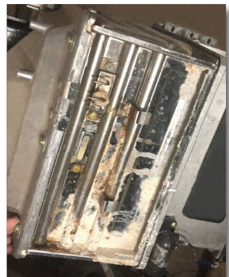
Lime scale buildup on a tankless water heater without ScaleRx ® protection in Phoenix, Arizona
