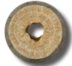
A cross-section of built up lime scale on the outlet of a water heater in Northern Illinois.
